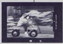
The electronic viewfinder: light emitting diodes tell you what the camera is doing automatically to give you correct exposure.
